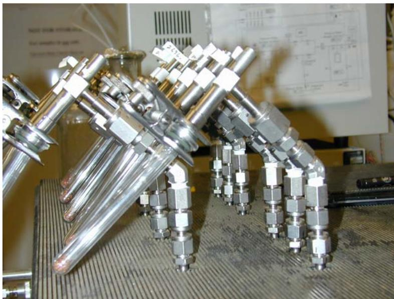
The bottom of the borosilicate glass is protected with a wad of clean copper turnings. This is a physical barrier to prevent glass against glass from scratching the bottom of the cracker tube. It also has the advantage of removing traces of H<sub>2</sub>S from sulphide bearing carbonates where the copper will turn a blackish colour. The change in colour is not necessarily a problem with future CO<sub>2</sub> samples. Change the copper when it is really discoloured.
