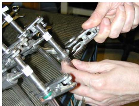
Place tube onto the cracker keeping the inner breakseal straight. When ready to crack, gently move the bottom front to back or side to side to release the gas. It should break easily if the etch is well done. After releasing the gas, leave the bottom joint in its final position (bent). **DO NOT STRAIGHTEN AFTER CRACKING THE TUBE.** This can damage the O-ring with a sharp glass edge rubbing onto it.
