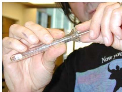
Pinch with thumb and finger against the edge of the female Rotulex joint
